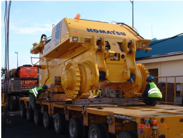
Image 13. Body of D 475 Bulldozer
