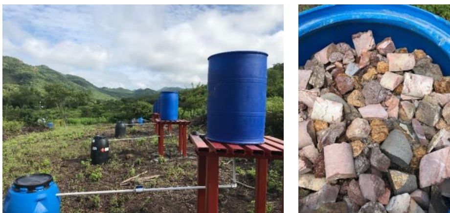
Photograph 3.1.1.5. a. Kinetic field test (left) and core samples in one of the reactors (right)
