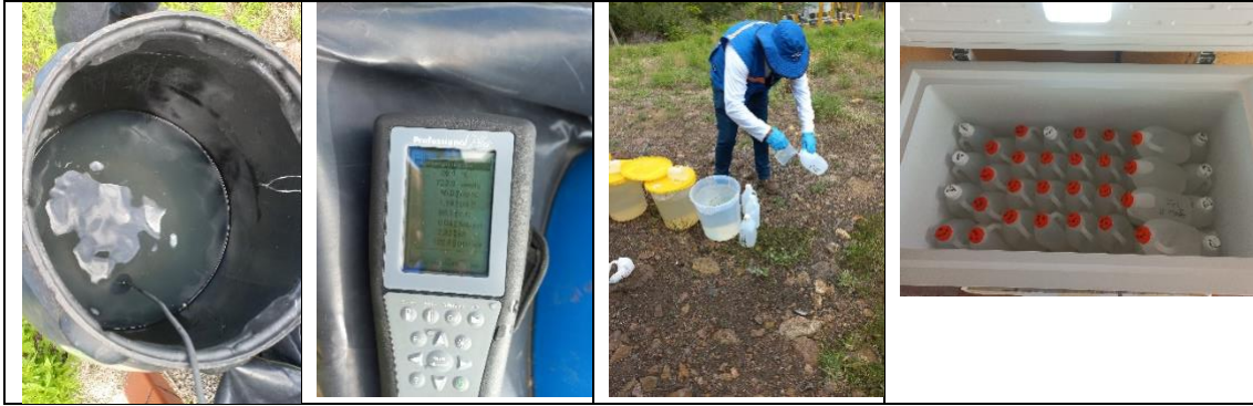
Pictures 2.6.1: measurement of physical parameters of water quality, collection, and storage of leachate volume.
