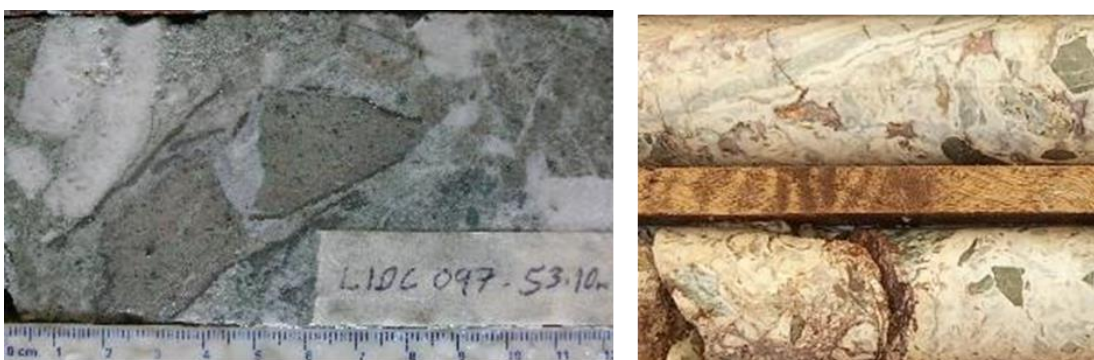
Figure 7-8: Central Breccia smectite altered clasts with sulphide rims cemented by quartz-calcite at 32.4 g/t gold and 19 g/t silver (left). Banded quartz-calcite vein at ~ 260 m below surface at 8.20 g/t gold and 52 g/t silver at the Cacao prospect (CCDC033-283 m; right).
