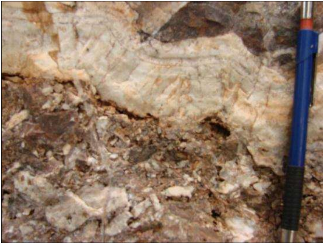
Figure 6-4: Close-up of part of La India Vein showing fault brecciated and re-sealed early emplaced vein (bottom) in contact with later banded quartz vein (top) (Source: Condor)
