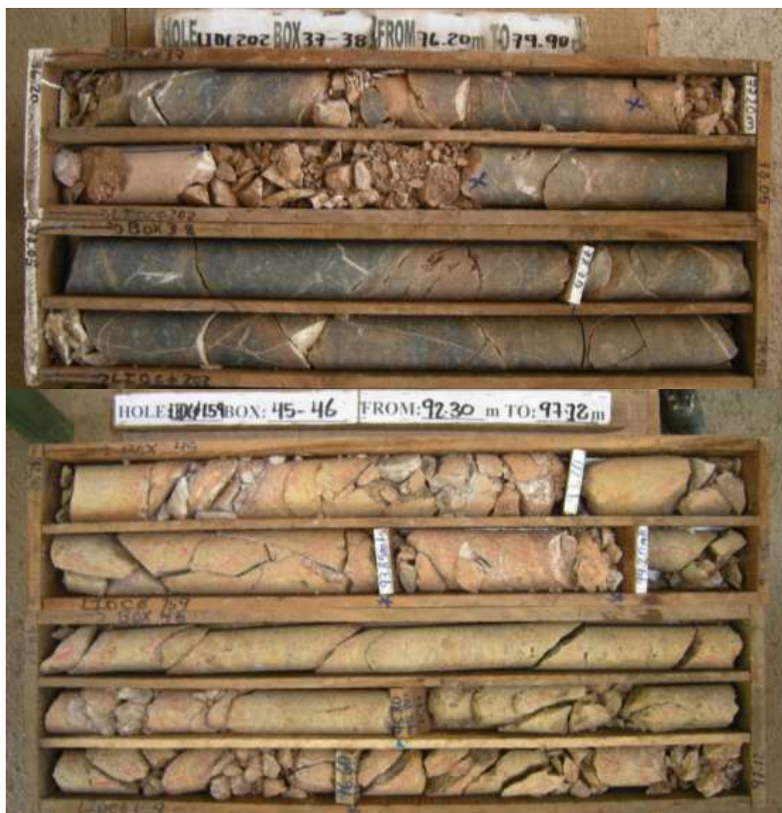
Figure 15-2: Hangingwall Core Intersections
