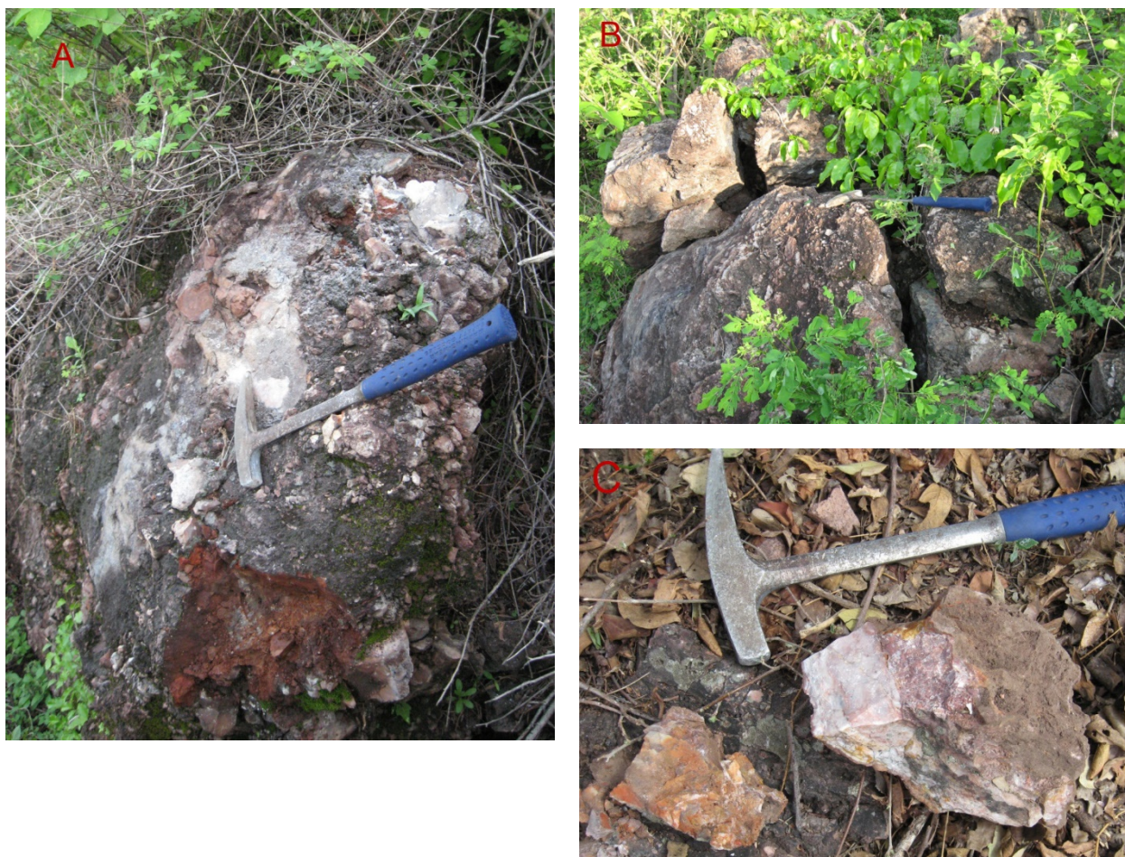
Photograph 6. A & B: Quartz cemented breccia, sample site 69016, 1.5 m; C: sample site 62185, 1 m @ 198 ppb Au.
