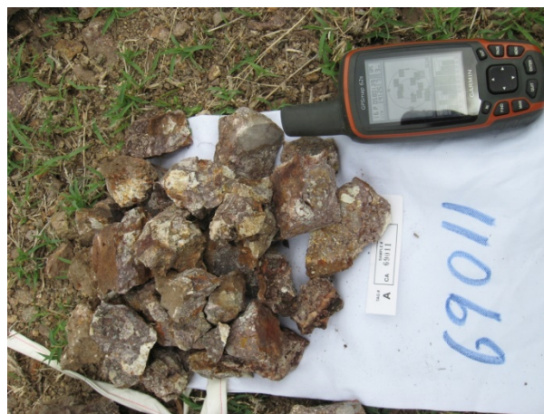
Photograph 12. Sample 69011: Au 270 ppb, As 28 ppm, Sb 12.8 ppm
