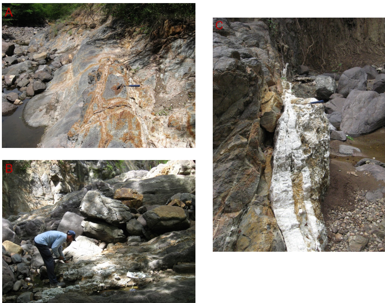
Photograph 10. Porphyritic andesite. A: fracture and calcite-quartz vein trend. B: Sample site 69050, 0.5 m quartz calcite pod among in zone of calcite quartz lined fractures and veinlets. C: NNW-SSE 20-60 cm calcite vein
