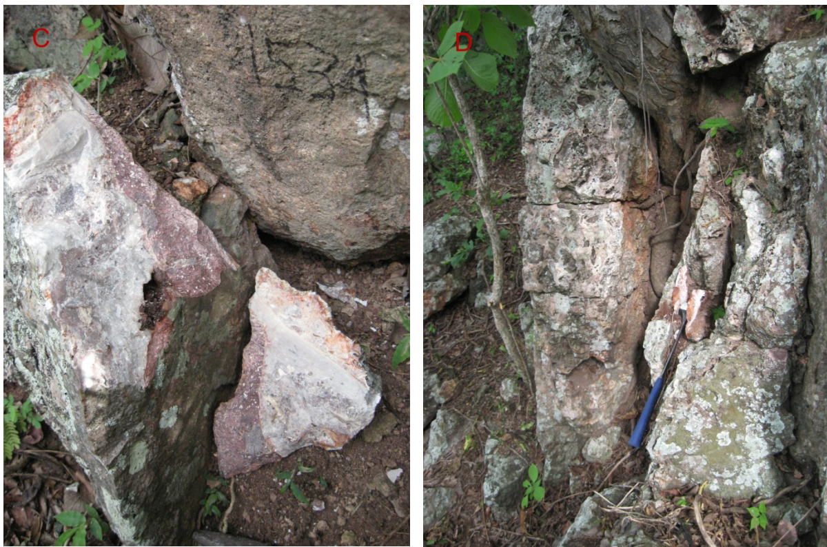
Photograph 4. A: main E-W vein at Santa Barbara; sample site 69033, 0.7 m @ 15.9 g/t Au; B: NW trending vein, sample site 69041, 0.5 m @ 3.1 g/t Au; C: sedimentary feature in NW vein; D: NW trending vein, quartz cemented breccia, rhyolite and quartz clasts
