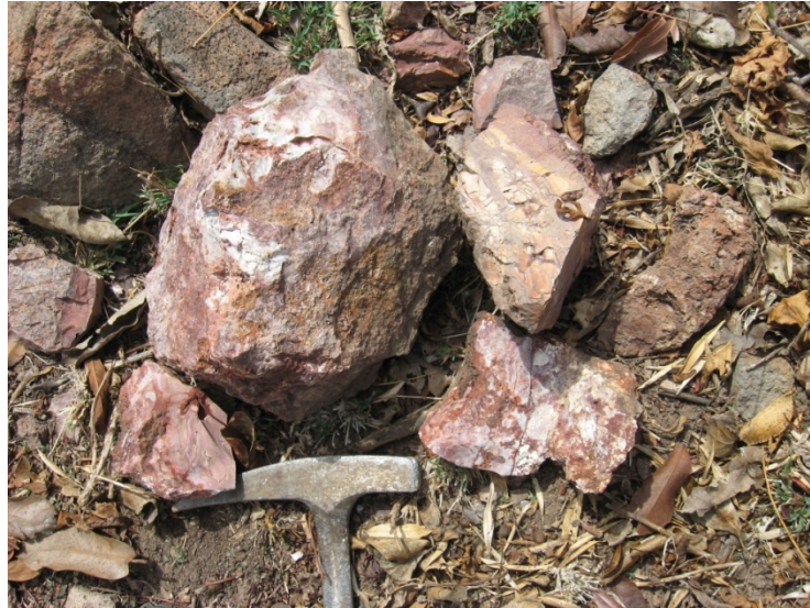
Photograph 14: float hematite stained siliceous breccia from trench area
