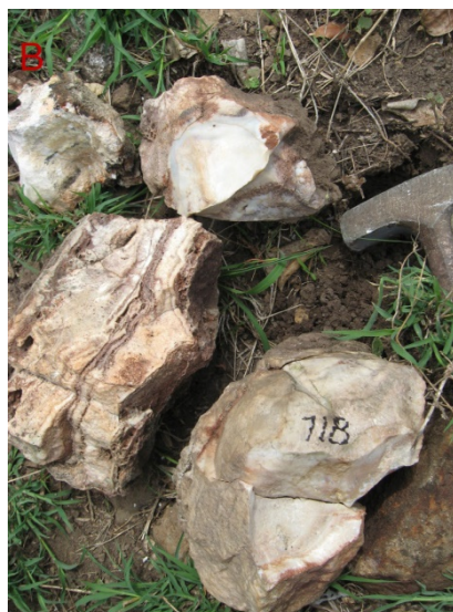
Photograph 16. A & B: massive to banded microcrystalline quartz and chalcedony; sample site 69012
