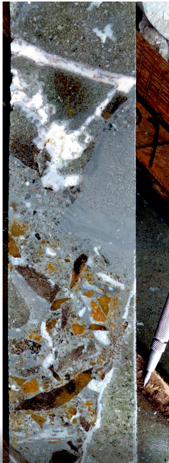
RIGHT. LIDC 099 @ 80.3 m Dyke of breccia, siliceous grey sediment (mudstone to coarse sandstone) with late coarse calcite fill.
