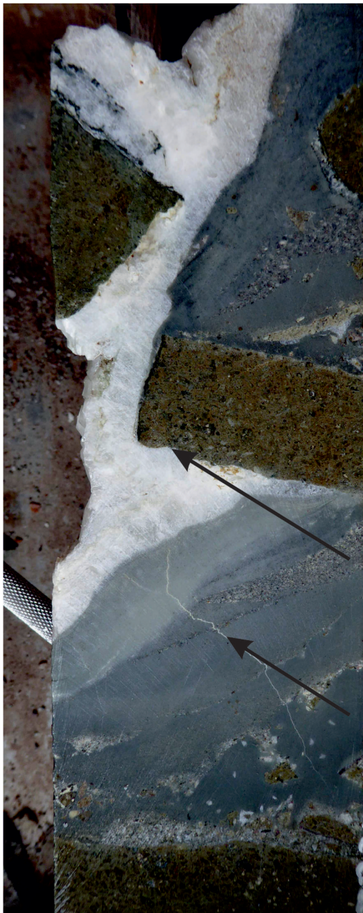
LEFT. LIDC 097 @ 146.2 m Dyke of siliceous grey sediment (mudstone to coarse sandstone) with late coarse calcite fill.
