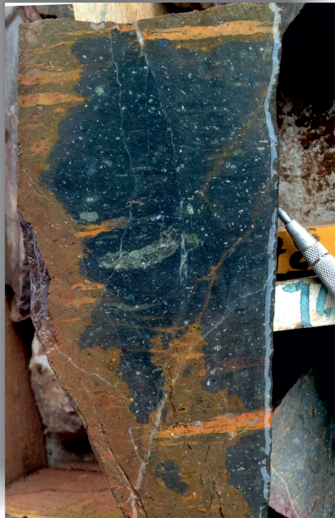
RIGHT. LIDC 313 @ 140 m Welded tuff with common large pumice fiamme. note contrast between weathered and non-weathered colours.
