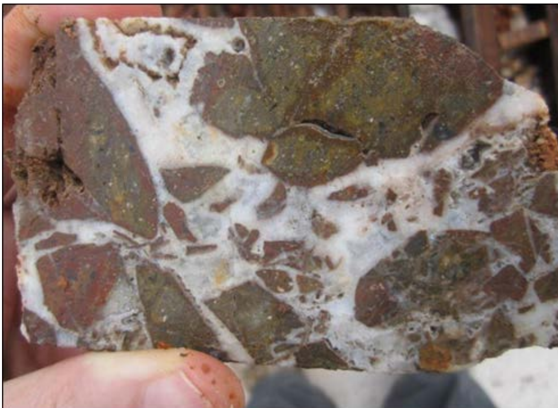
Figure 6-3: Gold Mineralised Breccia of the La India-California vein trend; image 1 (Source: Condor, June 2012)
