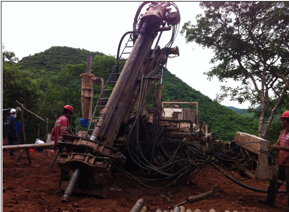
Figure 9-3: Rodio-Swissboring RC Drill Rig being set up during the 2012 Drill Program; June 2012
