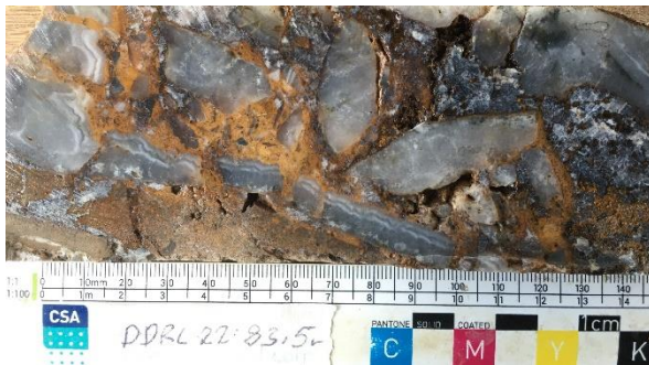
Figure 6. Left: Early banded amorphous grey quartz subsequently brecciated and infilled with silicified fault cataclasite (gouge).
