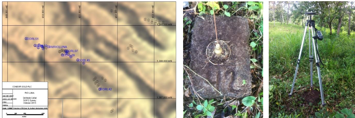
Figure 30. Map showing drillhole collar locations reported by First Point Minerals using GPS (black) and surveyed by Condor using DGPS (blue). Photographs of drillhole collar DDRL42 at the Santa Rita Prospect being surveyed by DGPS.
