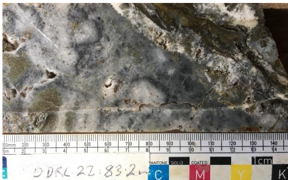
Figure 7. Left: Mixed (transitional) early amorphous grey quartz and saccharoidal white quartz with abundant disseminated and blebby sulphides. Right: High-grade transitional amorphous grey to saccharoidal white quartz vein with ghost bladed calcite replacement texture and disseminated sulphides that assayed at 57.6 g/t gold.
