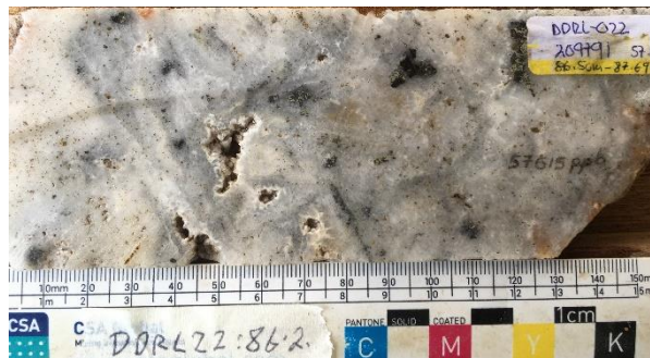
Figure 7. Left: Mixed (transitional) early amorphous grey quartz and saccharoidal white quartz with abundant disseminated and blebby sulphides. Right: High-grade transitional amorphous grey to saccharoidal white quartz vein with ghost bladed calcite replacement texture and disseminated sulphides that assayed at 57.6 g/t gold.
