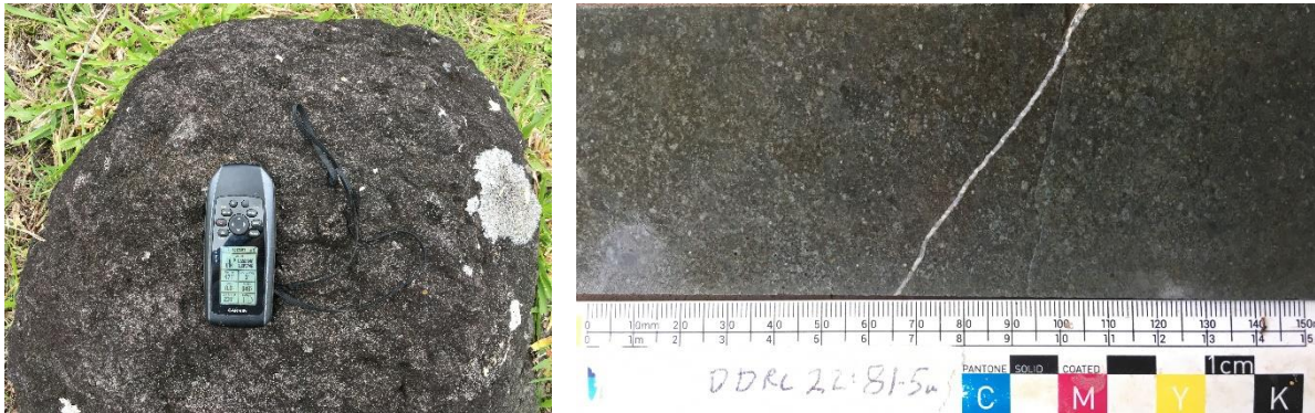
Figure 9. Left: Chlorite-calcite altered andesite tuff and fracture-fill calcite vein with disseminated fine pyrite selvage in outcrop (San Andres Prospect) and drill core (Balsamo East Prospect).
