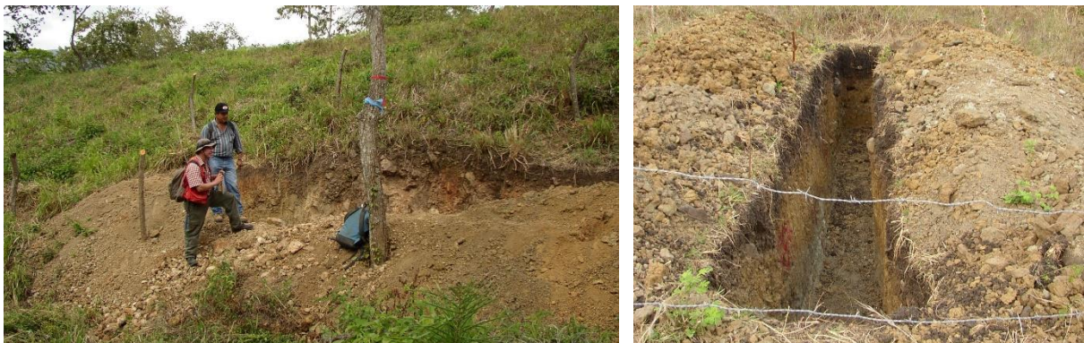
Figure 18. Trenches ready for sampling on sloping and flat land (from First Point Minerals presentation).
