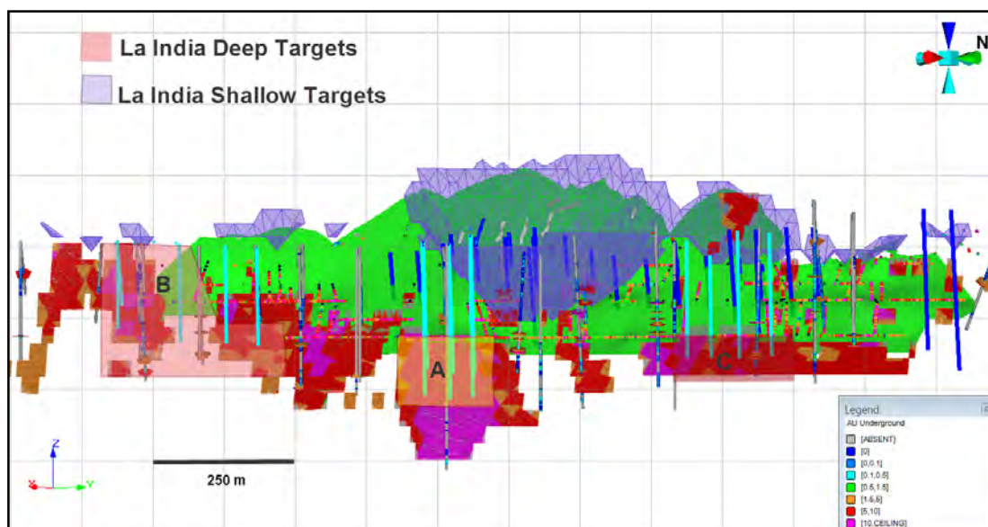
Figure 16-1: 3D View showing La India Exploration Targets - Dark Blue Holes show shallow drilling targeting up-dip extension of California Vein, Light Blue indicate Deeper drilling to increase the confidence in estimates at depth
