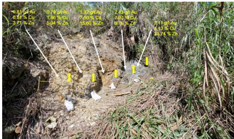
Figure 3: Trenching results taken across a 5 metre outcropping zone of mineralisation within the historical Keon open pit mine.
